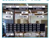
**PTZ protocol analyser** can be used inline to troubleshoot keyboard controllers and cameras.
