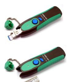
With a LC / SC patch cord, the Light Source can be used for most widespread fiber interfaces such as LC / ST / SC / FC connectors. It is suitable to test both Singlemode and Multimode cables.
