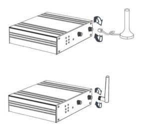
**NOTE:** NR300 router supports dual antennas with MAIN and AUX connectors. MAIN connector is for data receiving and transmission. AUX connector is for enhancing signal strength, which cannot be used separately.
