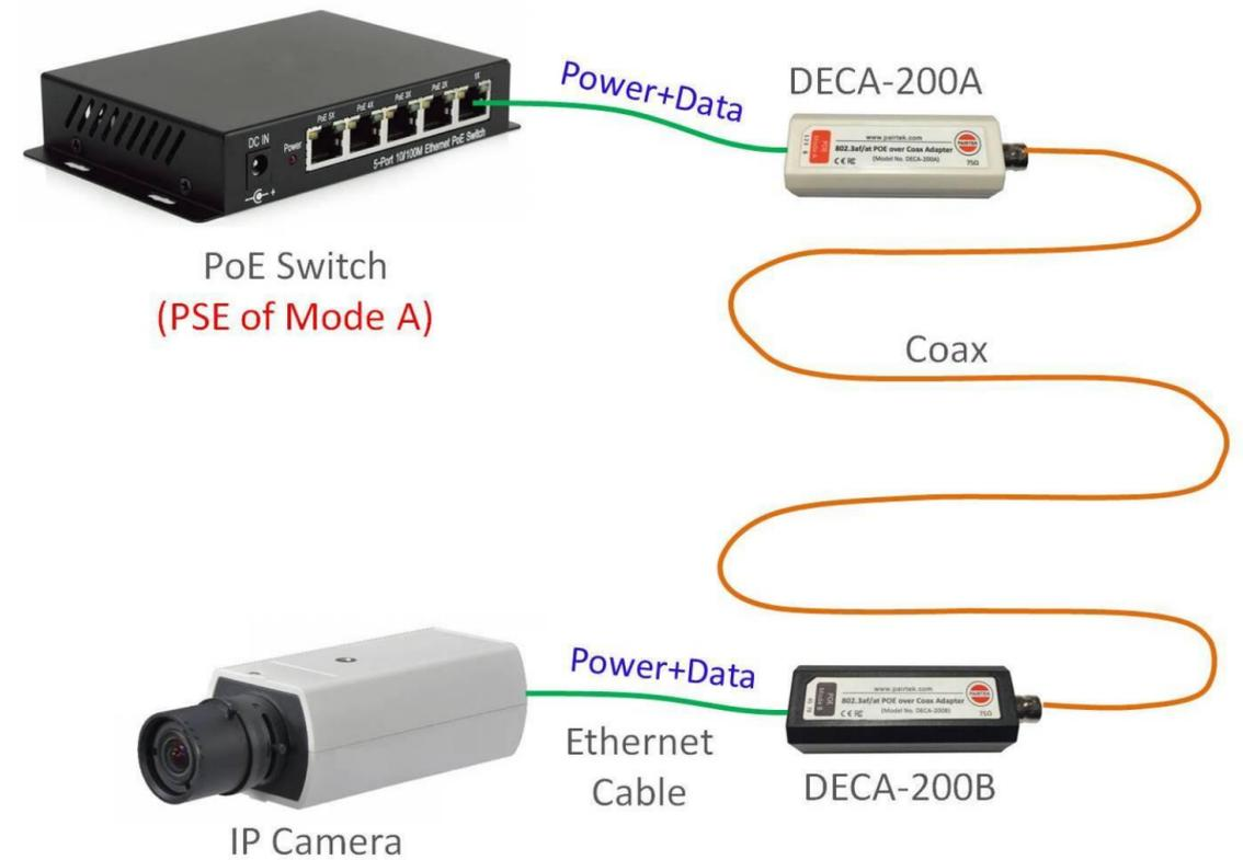
FIG.1 Set up of PoE-over-Coax Adapter Kit with a PSE of Mode A
