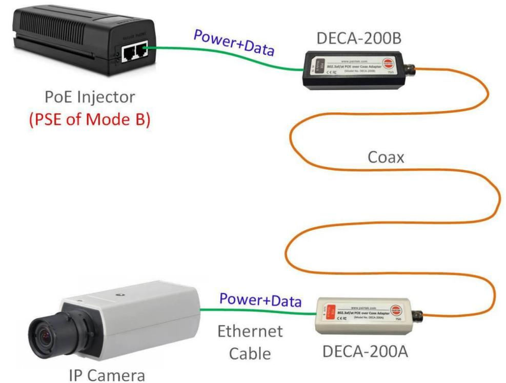
FIG.2 Set up of PoE-over-Coax Adapter Kit with a PSE of Mode B
