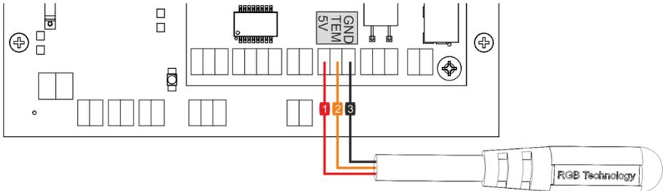
fig. 7 Temperature probe and clock wiring diagram
