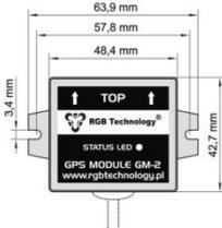
fig. 4 Receiver module GPS GM-2 – overall view
