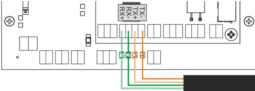
Fig. 3 LAN and clock wiring diagram
