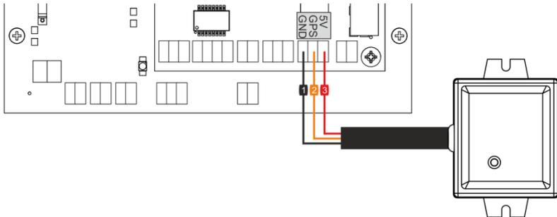
fig. 6 Connection the GPS module to the clock
