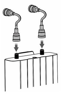
(2) Attach the wireless bridge to the antenna.
