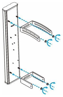
(2) Secure the two fastening pieces to the upper and lower brackets with four screws, two for each.
