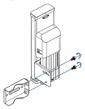
(3) Secure the antenna to the pole.
