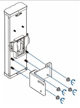
(2) Attach the bracket holder to the bracket with two screws.
