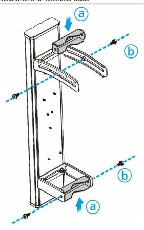
(3) Secure the antenna to the pole.
