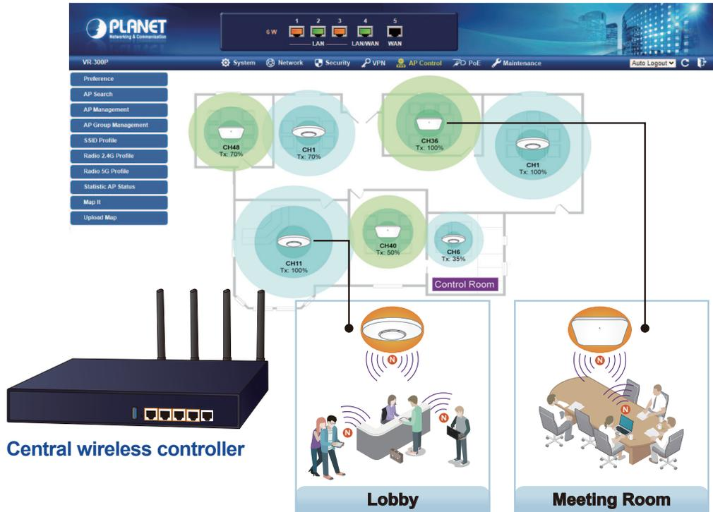
For example, to configure multiple Smart APs of the same model, the VR-300W5 and VR-300PW5 allow clustering them to a managed group for unified management. According to requirements, wireless APs can be flexibly expanded or removed from a wireless AP group at any time. The AP cluster benefits bulk provision and bulk firmware upgrade through single entry point instead of having to configure settings in each of them separately.
