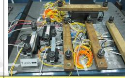
Sinusoidal Vibration Test--X axis Mechanical Shock Test: ±X axis
