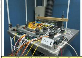
Sinusoidal Vibration Test--Z axis Mechanical Shock Test: ±Z axis
