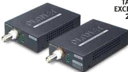
PLANET Long Reach PoE solution is designed to extend IP Ethernet transmission and inject power simultaneously into a remote 802.3af/at PoE compliant powered device (PD) beyond the 100 meters distance limit of Ethernet.
