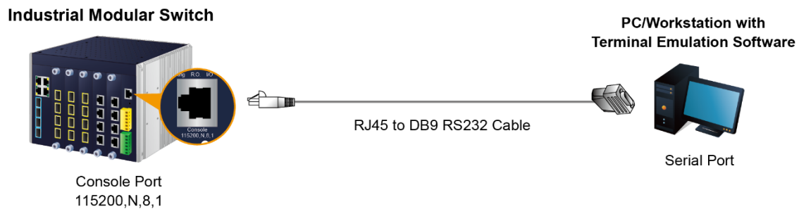
Figure 3-3-1: RJ45-to-DB9 console connection
