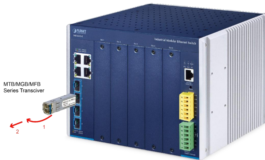
Figure 2-3-2: Pull out the SFP/SFP+ Transceiver Module
