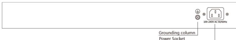
**Note:** This device relies on the separate protective earthing terminal. The device installation shall be permanently connected to building earth by a skilled person.
