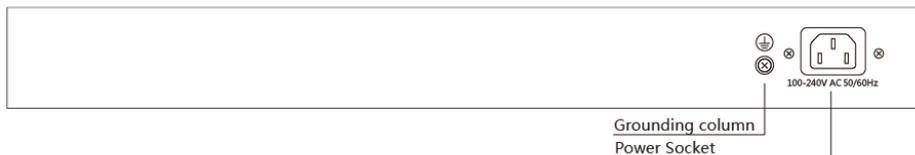
**Note:**This device relies on the separate protective earthing terminal. The device installation shall be permanently connected to building earth by a skilled person.
