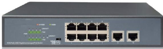
20117390 contains 10 RJ45 ports and 1~8 support PoE functions. The PoE ports can automatically detect and supply power to IEEE802.3af/at compliant Powered Devices (PD). The electrical power and data transmission on the same cable can expand your network to the places where no power lines or outlets, where you can install devices such as APs, IP cameras, or IP phones etc.
