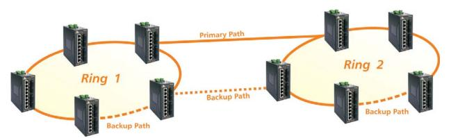
methods between network rings. Therefore, all the switches do not have to be confined and connected in one big ring. A network containing numerous switches can be broken into smaller, more manageable rings to ensure network efficiency and performance.
