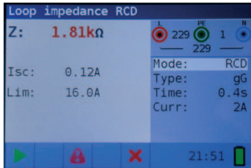
Figure 4 25: Example of fault loop impedance measurement results using trip-lock function
